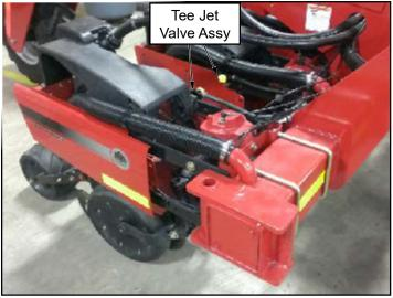
FIG. # 5-39 Tee Jet Valve Assy
