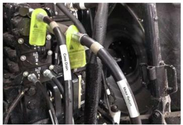
FIG. # 3-3 Motor Return Line, and Fan Motor Case Drain Line Connected
